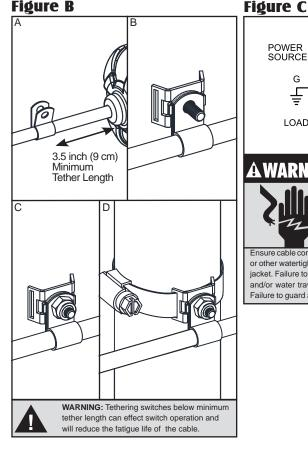
Due to weight of cable, pumping range above horizontal is NOT equal to pumping range below horizontal. Use values published on front page as a guide. Pumping ranges are based on testing in non-turbulent condi tions. Range may vary due to water temperature and cord shape. Note: As the tether length increases, so does the variance of the pumping range.
