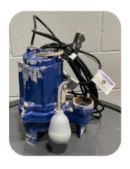
This JMI Submersible Sewage Pump ran for more than 250,000 cycles in the onsite JMI Proving Grounds. The 9S-JMI and switch still met performance specifications upon test completion.
