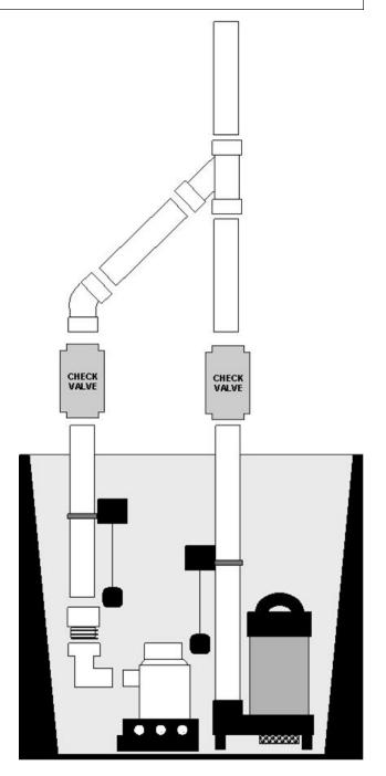
3. Make sure that the float ball on the backup switch will not get caught or hung up on the primary pump or any other object that will restrict the switch from turning on.
